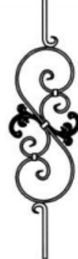
EIW 141 □12-16 / Ø14mm SCROLLS : 16 x 8 / LEAF CAST 580 H x 215 W HEB / PL
