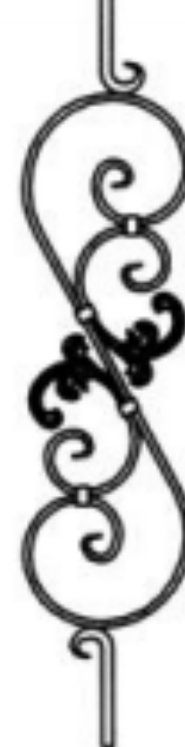
EIW 140 □12-16 / Ø14mm SCROLLS : 16 x 8 / LEAF CAST 690 H x 215 W HEB / PL
